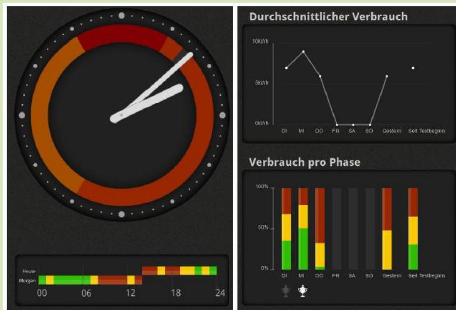
The display on the left shows in the outside ring of the analogue clock whether it is favourable to consume energy in the next 60 minutes (top) and the forecasted favourability for the next 24 hours (bars below). The display on the right shows the average consumption of the last week (top) and the consumption within the different price levels (bottom).<sup>10</sup>
