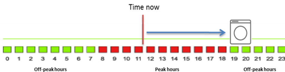
Figure 2: Scheduling of the appliance operation with respect to the price of electricity Source: RSE internal documentation
