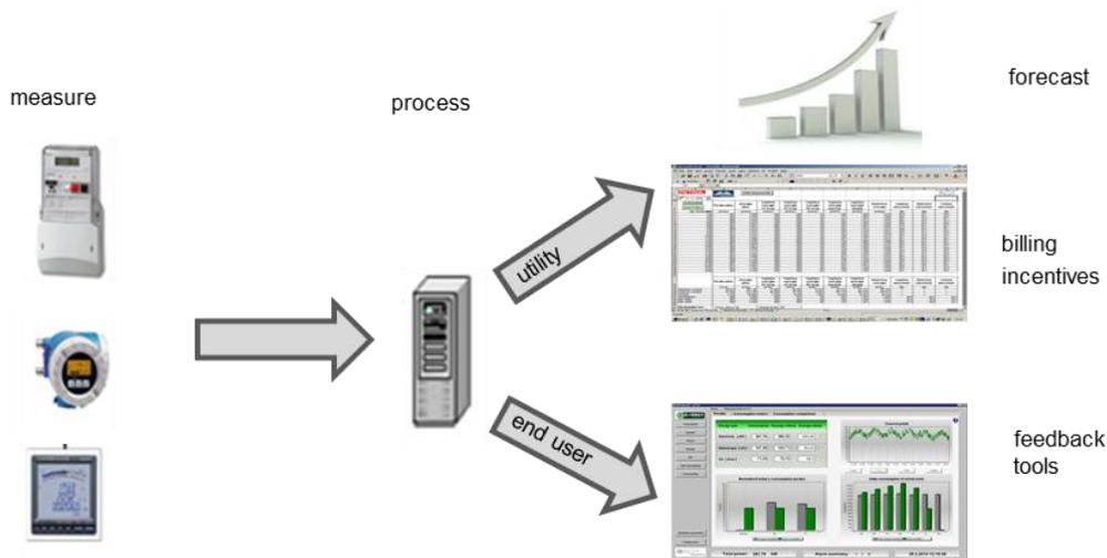
Figure 2: Monitoring process scheme (source: KIBERnet documentation)
