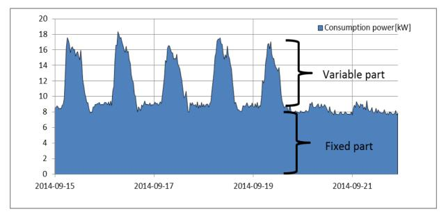
Figure 2: Example of electricity consumption in a commercial building: consumption history for 1 week [measurements from the commercial building, project SPEU]
