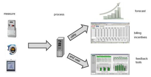
Figure 2: Monitoring process scheme (source: KIBERnet documentation)
